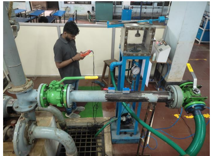
Fig3.1.9 Operator using an ultrasonic flow meter and sensors mounted on the pipe.
