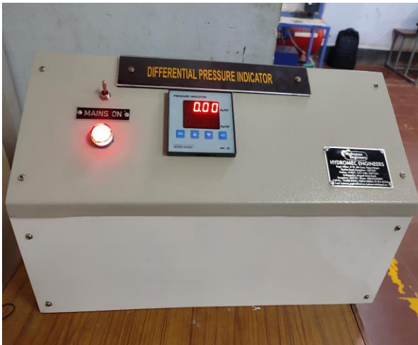
Fig 3.1.6 Differential Pressure Gauge.
