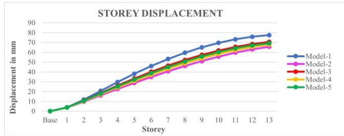
Chart -5: Storey displacement variation in X-dir. for various types of bracings on FGS
