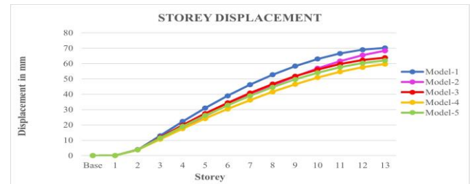
Chart -8: Storey displacement variation in Y-dir. for various types of bracings on SGS
