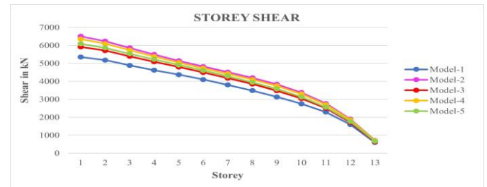
Chart -14: Storey Shear variation in Y-dir. for various types of bracings on FGS
