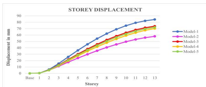
Chart -7: Storey displacement variation in X-dir. for various types of bracings on SGS
