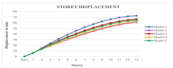
Chart -6: Storey displacement variation in Y-dir. for various types of bracings on FGS
