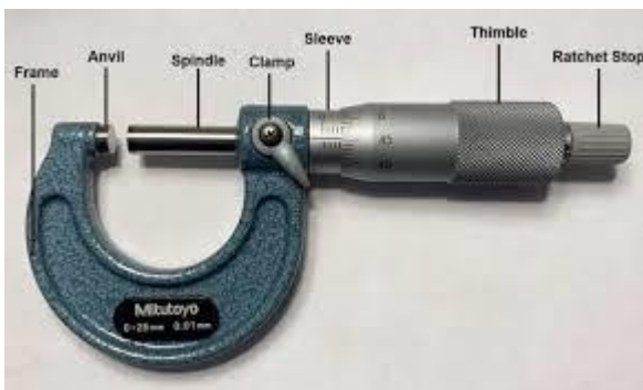
Fig 2: Micrometer
